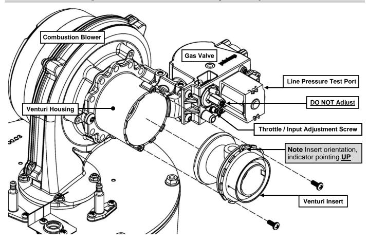
Figure 1-1 LP-Venturi Insert and Throttle/Input Screw Adjustment
