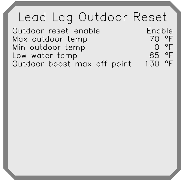
Figure 2-17 LL Outdoor Reset Screen
