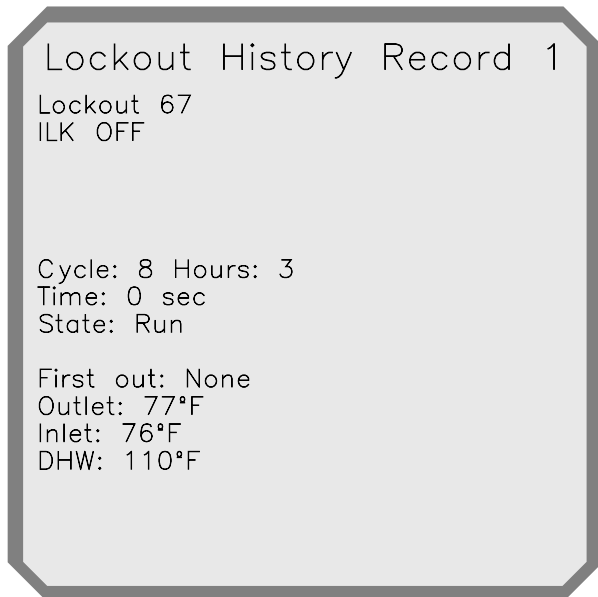
Figure 2-31 Example Lockout History Record Screen
