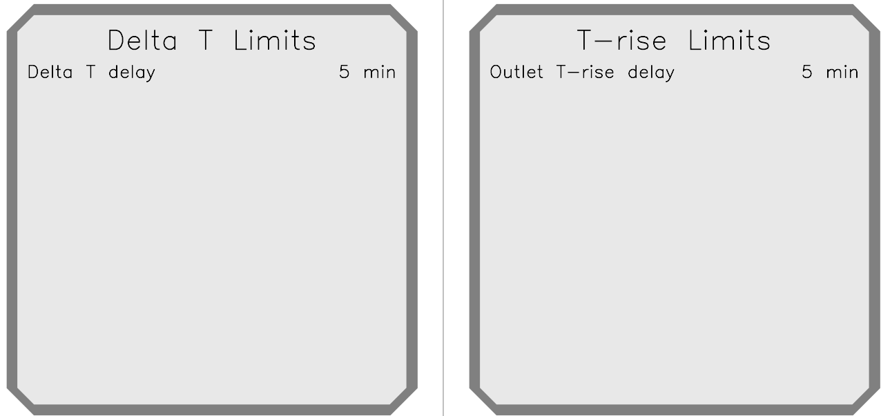
Figure 2-25 Delta T & T-rise Limits Screens
