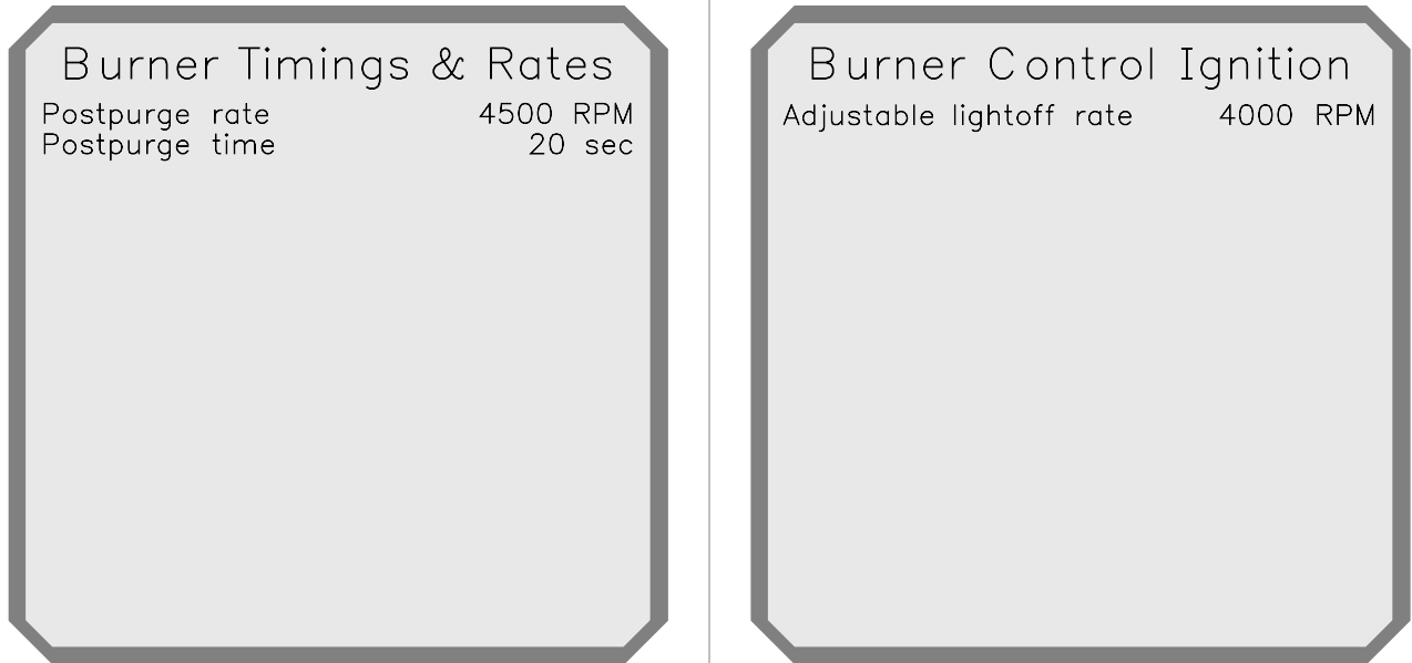
Figure 2-27 Burner Control Ignition and Timings & Rates Screens
