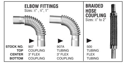
**INSTALLATION INSTRUCTIONS:** Clean fittings before soldering. Use non-acid (rosin) flux. Install Fast/Flex so that expansion or vibration movement will be at right angles to the flex section, and will not subject it to "accordion action." Avoid outside abrasion of the flex section. Do not twist hose when tightening threaded fittings.
