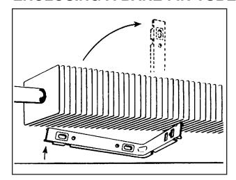
**AC ADAPTER BRACKET** — Sometimes it's necessary to add an enclosure to previously-installed bare fintube. AC adapter brackets make this a simple job.
