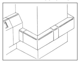
**COLUMN COVER SET** — Use to conceal bare or insulated piping which runs around a column. Available in heights of 5", 11" and 16", for 1 tier, 2 tier and 3 tier installations.
