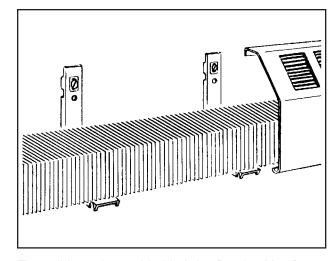
They slide under and behind the fin-tube. You fasten them to the wall and snap on any Slant/Fin enclosure instantly.
