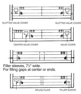
Splice plates, 3" wide, are used for narrower gaps.
