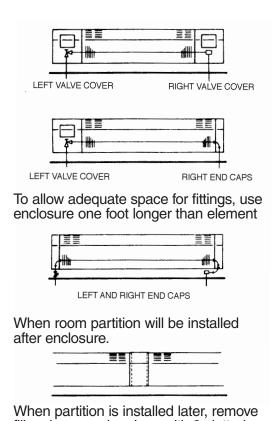
filler sleeve and replace with 2 slotted end caps.
