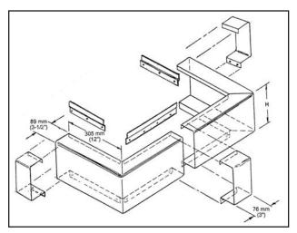
Set consists of 2 ea. 12" x 12" L-shaped sections, 3 ea. 3" telescopic splice plate, 4' of hanging strip and 20" of rubber gasketing. Will accommodate columns up to 14" deep (to face of radiation enclosure) and up to 25" wide; may easily be trimmed to suit smaller dimensions.
