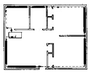
First take wall to wall measurements of all rooms from the plan or by actual field measurement. Next. calculate the heat loss for each room, using the IBR or equivalent method. Then translate the output required into the list of materials needed for each room and wall.
