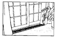
HYDRONIC FLOOR BOX HEATER recesses neatly into the floor for uninterrupted heating comfort at patio doors and floor length windows. Ask for publication HFB-10
