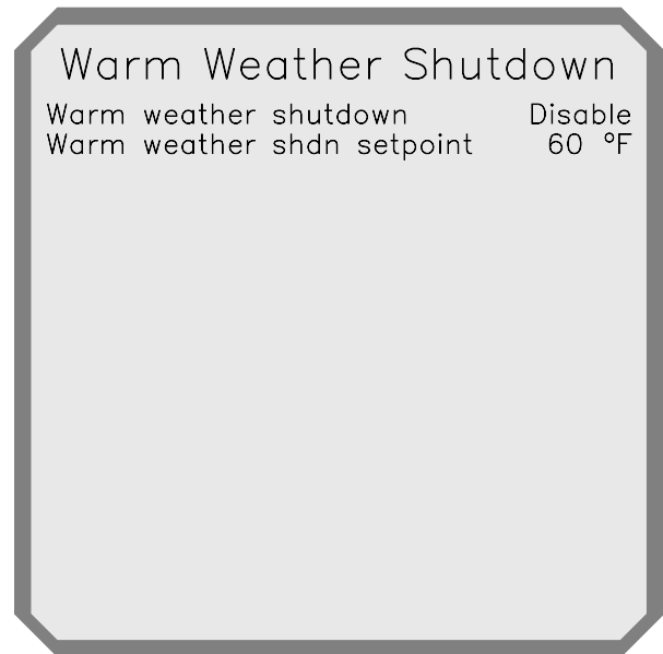
Figure 2-12 WWSD Configuration Screen
