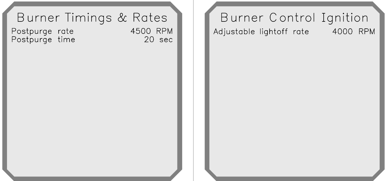
Figure 2-27 Burner Control Ignition and Timings & Rates Screens
