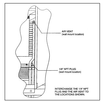
Figure 2. Air vent installation
