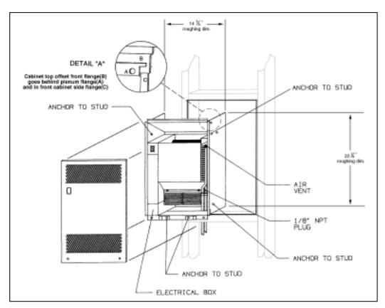
Figure 4. Wall installation
