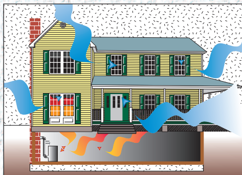
Ordinary boilers consume warm household air which causes infiltration of chilly outdoor air to replace it.
