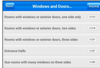
Infiltration Factor – Windows and Doors
