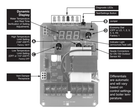
**NOTE:** Settings can be checked using the TEST/SETTINGS Button. See page 11 for details.
