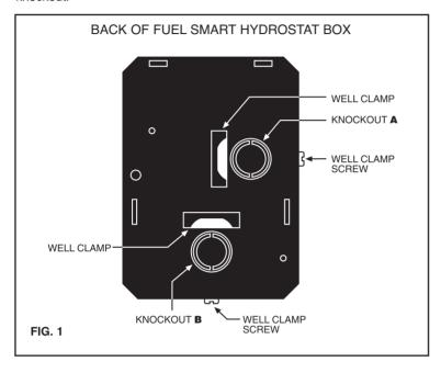
**STEP 2** Place control on the well. While holding box against well nut, tighten well clamp screw. (Fig. 2)
