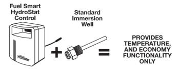
When installing on a standard immersion well, the LWCO function should be turned off (see page 9 for instructions). A buildup of heat transfer grease or other coatings in older wells can interfere with continuity between the sensor and the well causing a false low water shutdown. Turning off the LWCO function will prevent this from occurring.
