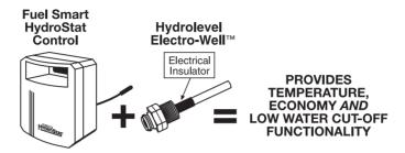
When installed on an Electro-Well<sup>™</sup> (sold separately), the Low Water Cut-Off function is automatically activated. Heat transfer grease should not be used. **NOTE:** For proper operation, there must be 1/2" clearance between the copper well tube and any furnace within the boiler.
