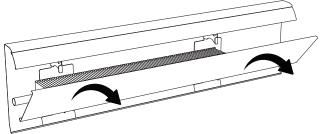
3. Remove any existing damper sections.
